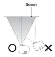
Set up so that the projector is parallel to the screen. If the projector is set up at an angle to the screen, distortion of the images will occur.
